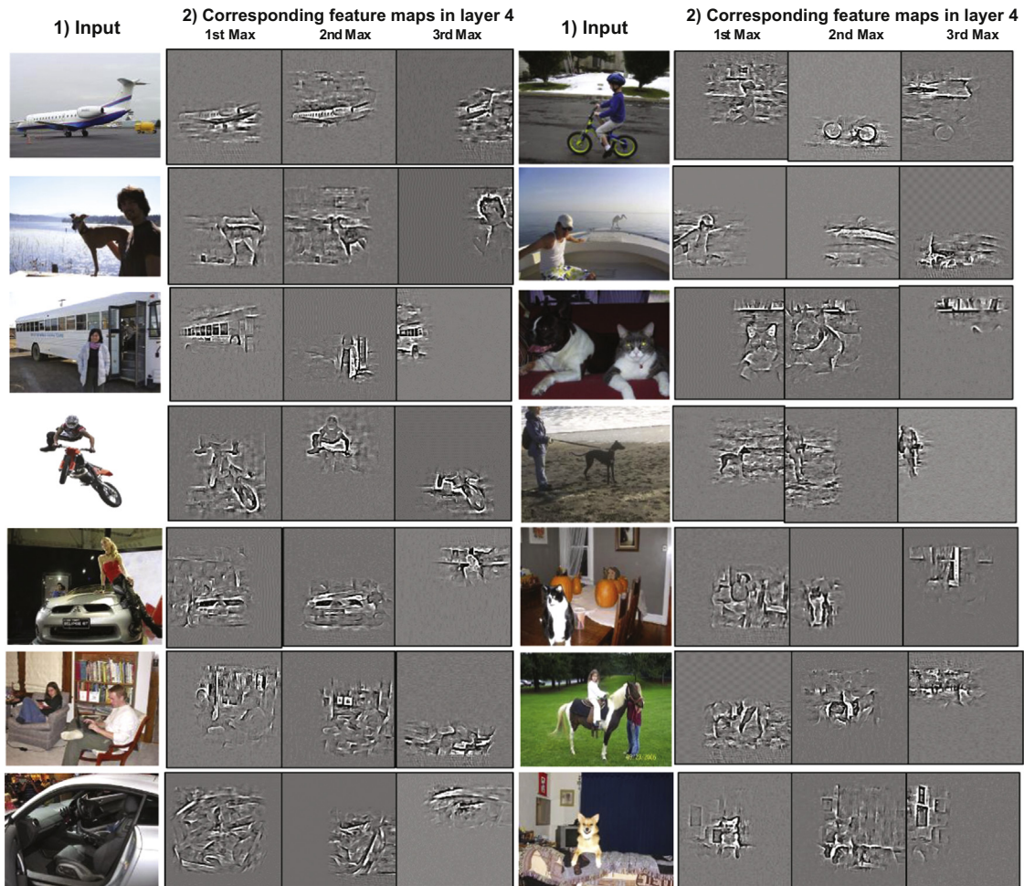
Fig. 4. Visualization of the feature maps in layer 4 when inputting a raw image. (1) Examples of input images. (2) Corresponding largest 3 feature maps in layer 4, visualized by reconstructing the feature maps in the 4th layer into the input space.
